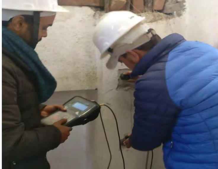
Figure 18: Photograph showing Schmidt Hammer Test
