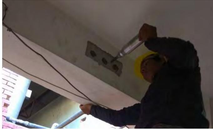
Figure 17: Photograph showing Schmidt Hammer Test
